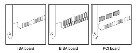
An ISA board has a single row of contacts along its connectors. There is usually a single notch in the connector.
